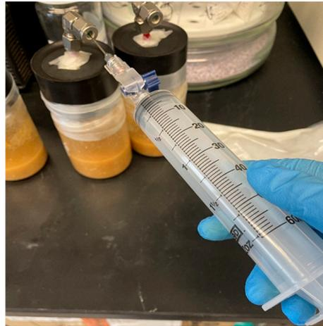
**Figure 3.** Biogas withdrawal from anaerobic digester.
