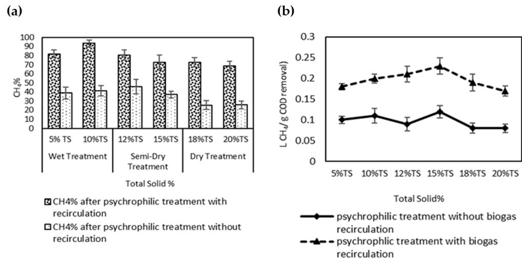
**Figure 4.** (a) Impact of total solid percentages and recirculation of biogas on methane concentrations in the biogas (b) Variation of methane yield with different total solid percentages.
