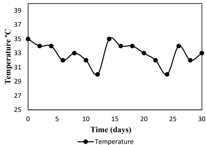
**Figure 6.** Temperature profile during anaerobic treatment of food waste.
