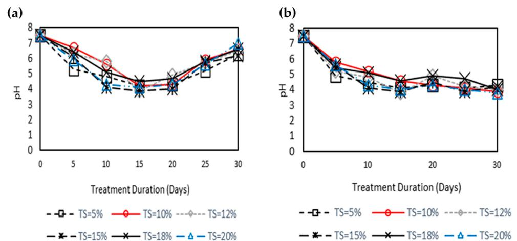
**Figure 7.** pH profile during anaerobic treatment. (a) with recirculation of biogas, (b) without recirculation of biogas.
