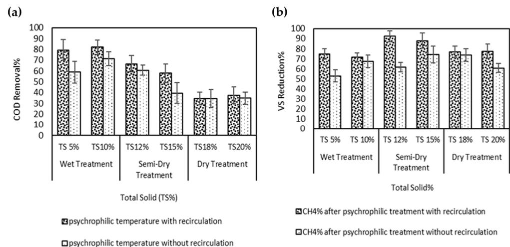
**Figure 5.** (a) COD removal efficiency and (b) VS reduction by anaerobic treatment with or without recirculation of biogas.
