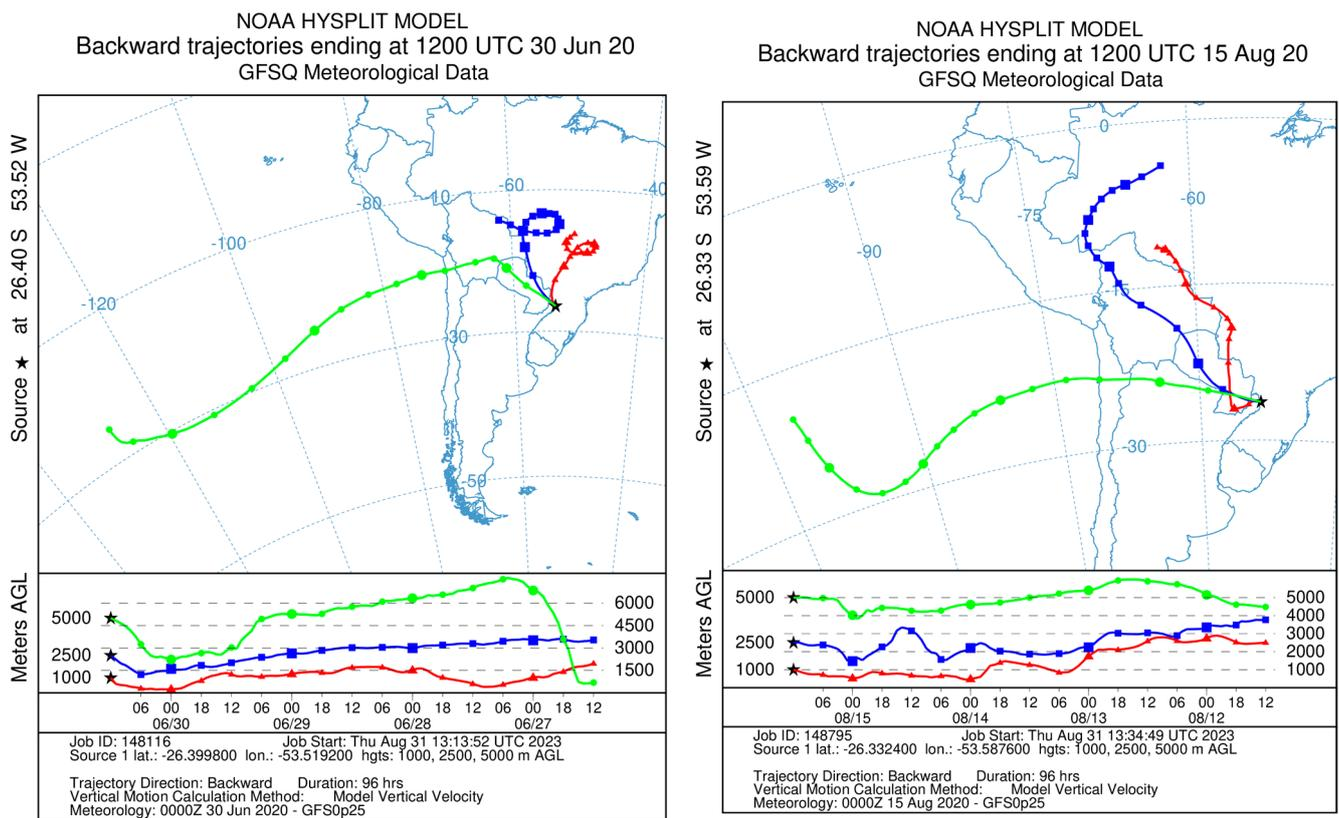
**Figure 2.** Ninety–six hours of backward trajectories modelled by HYSPLIT for the two air masses sampled in the study. Line colours indicate different altitudes of air masses: red line represents 1000 m, blue line refers to 2500 m, and green line represents 5000 m. Each point on the trajectory represents a period of 6 h.
