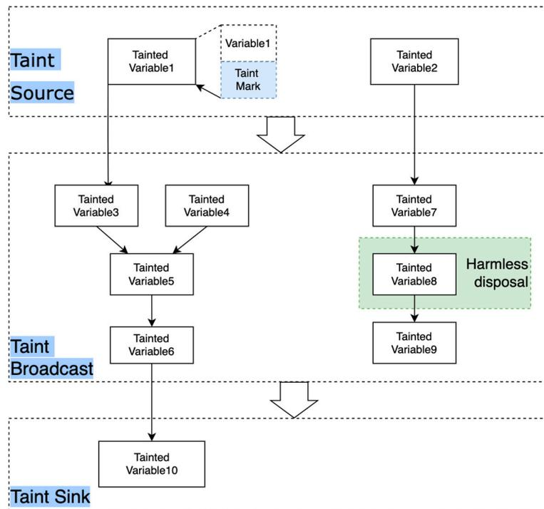
Figure 5. Schematic diagram of three steps in the taint analysis process.
