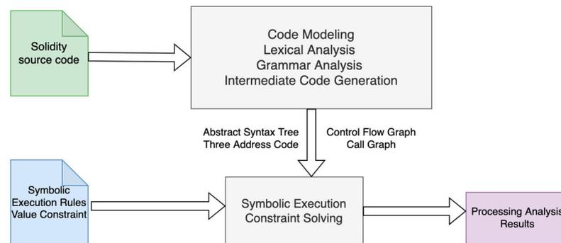
**Figure 3.** The process of symbolic execution technology for vulnerability analysis.
