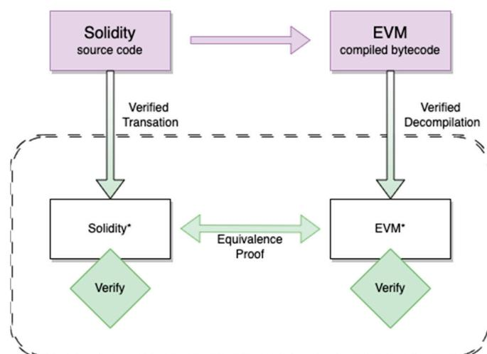
**Figure 2.** The conversion process of solidity code and EVM bytecode in formal verification.
