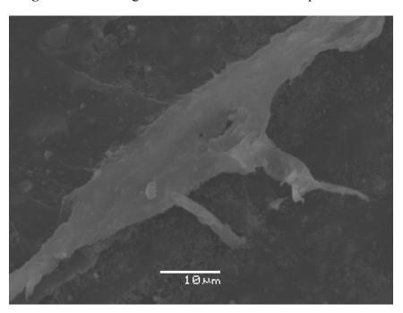
Figure 8. SEM image of the macro-crack on test specimen B5.
