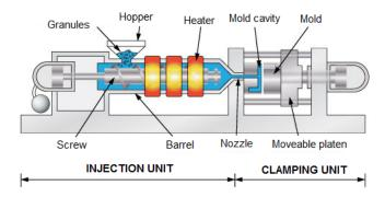
One of the main advantages of the injection molding process is the fact that it allows the high-volume manufacturing of plastic products. Often the geometric form of such products is very complex and must meet narrow tolerance requirements. This is especially true in those cases where different thermoplastic materials that have different shrinkage values are used.
